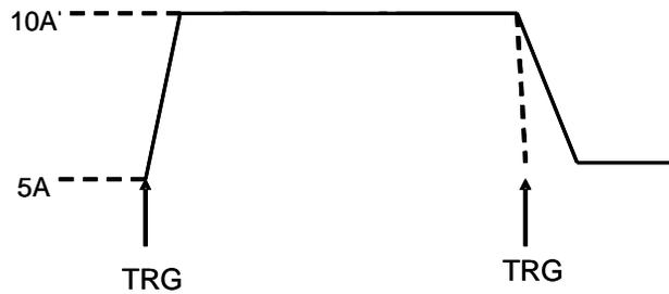
Picture 4.12 Trigger Operation Mode
