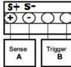
The following shows wiring diagram for the remote sensing:
