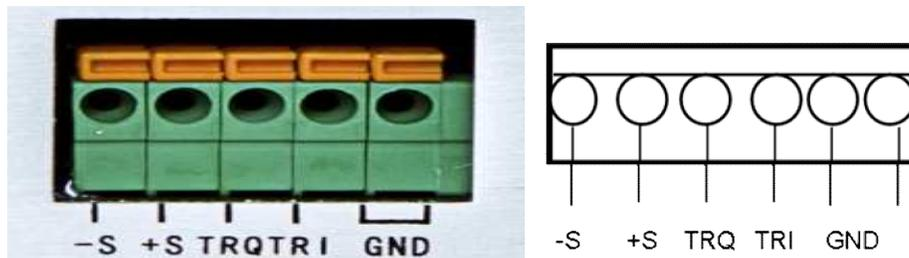
Picture4.4 Remote Measurement Terminals
