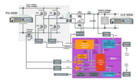
Figure 6:Test Setup, Simplified
