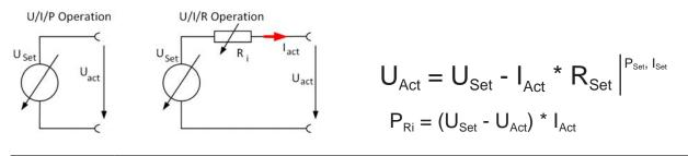
With resistance mode being activated the function generator will be unavailable and the actual power value provided by the device does not include the simulated power dissipation of Ri.
