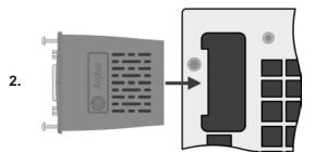
Insert the interface module into the slot. The shape ensures correct alignment.
