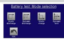
There is a choice between modes "Static discharge" (constant current), "Dynamic discharge" (pulsed current), "Static charge" (constant current) and "Dynamic test" (flow of charge/discharge).
