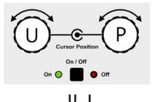
The physical quantities on the depiction of the knob show the current assignment. The left knob is always assigned to the voltage (U), while the right knob can be switched by tapping on the depiction.
